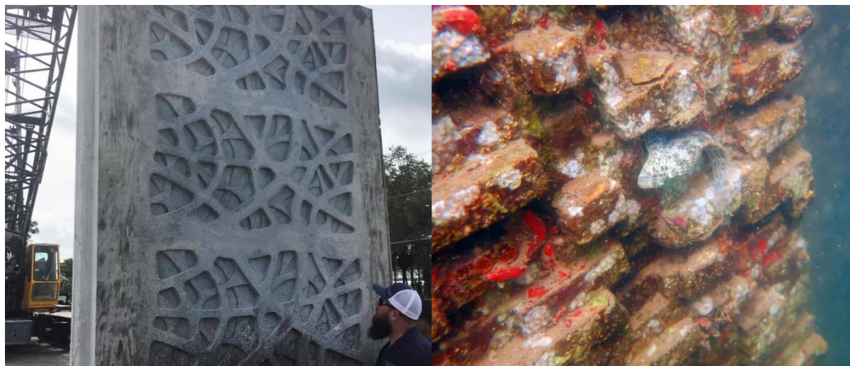
Figure 3-5: Example of Concrete with Biologically Sensitive Admixtures and Surface Complexity (EConcrete, 2023)
